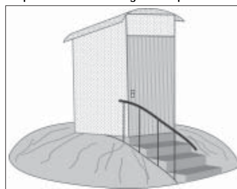
Raised Pit Toilet (Shared)
